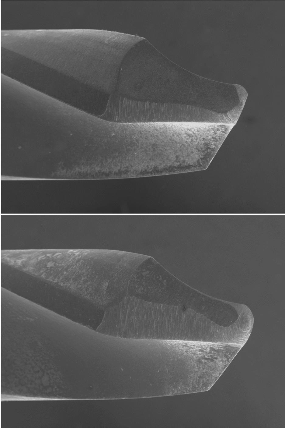
The image on top is a cycled drill bit, while the image below is a non-cycled drill bit. In the graphs below, the orange data points represent the cycled drill bits, while the blue data points represent non-cycled drill bits.
