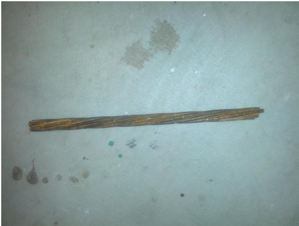
Untreated Wire Rope following 100 hours exposure in salt spray chamber
