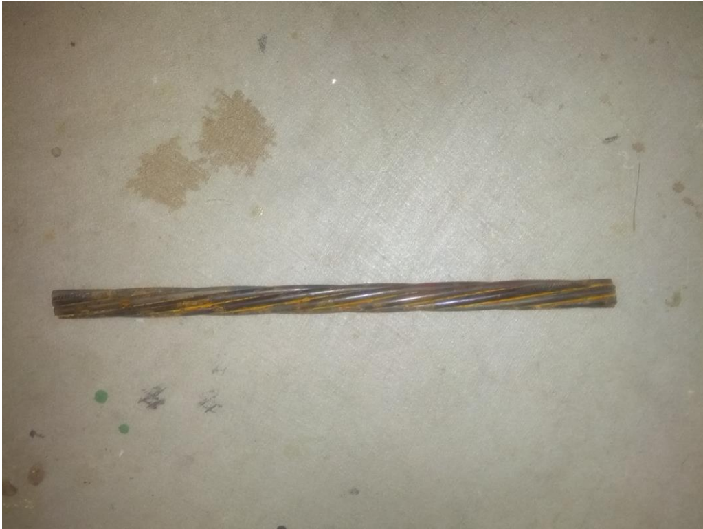
Treated Wire Rope following 100 hours exposure in salt spray chamber
