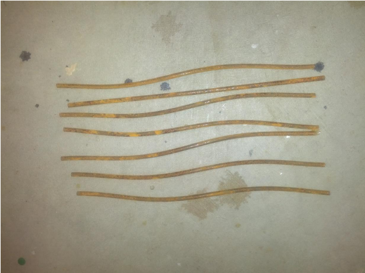
Untreated Wire Rope with Strands Separated
